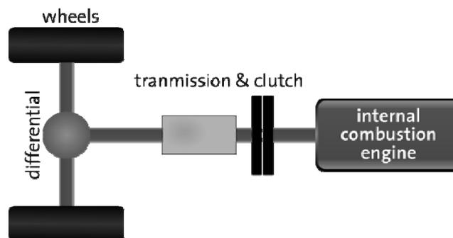
Figure 2: schematic representation of a conventional powertrain
