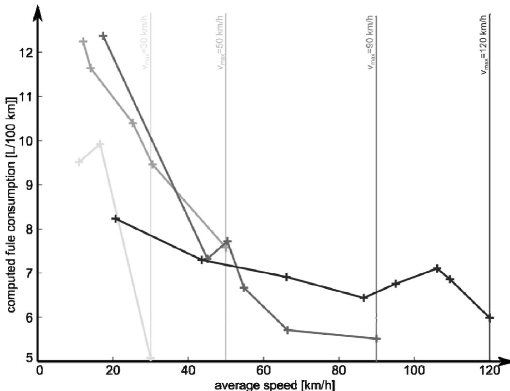
Figure 6: fuel consumption for a 1500 kg, 80kW conventional vehicle
