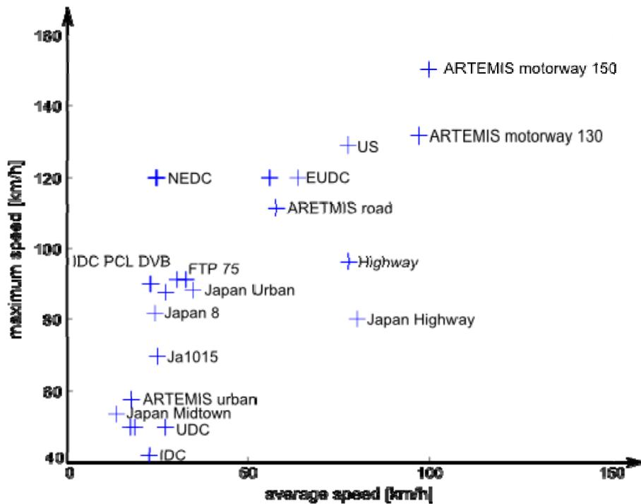
Figure 5: spread in a maximum-speed / average-speed classification scheme
