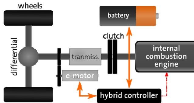
Figure 3: powertrain layout of a parallel hybrid
