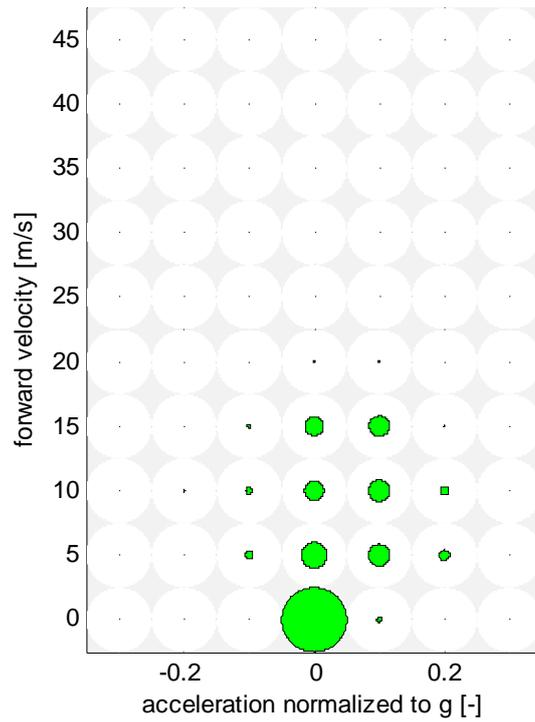
Figure 4: example of drive cycle characterization using the kinetic parameters described in [10] (here on ARTEMIS urban). Note that the circles represent the probability of having some acceleration at a known speed, relative to the most likely condition – in this case no acceleration at standstill.
