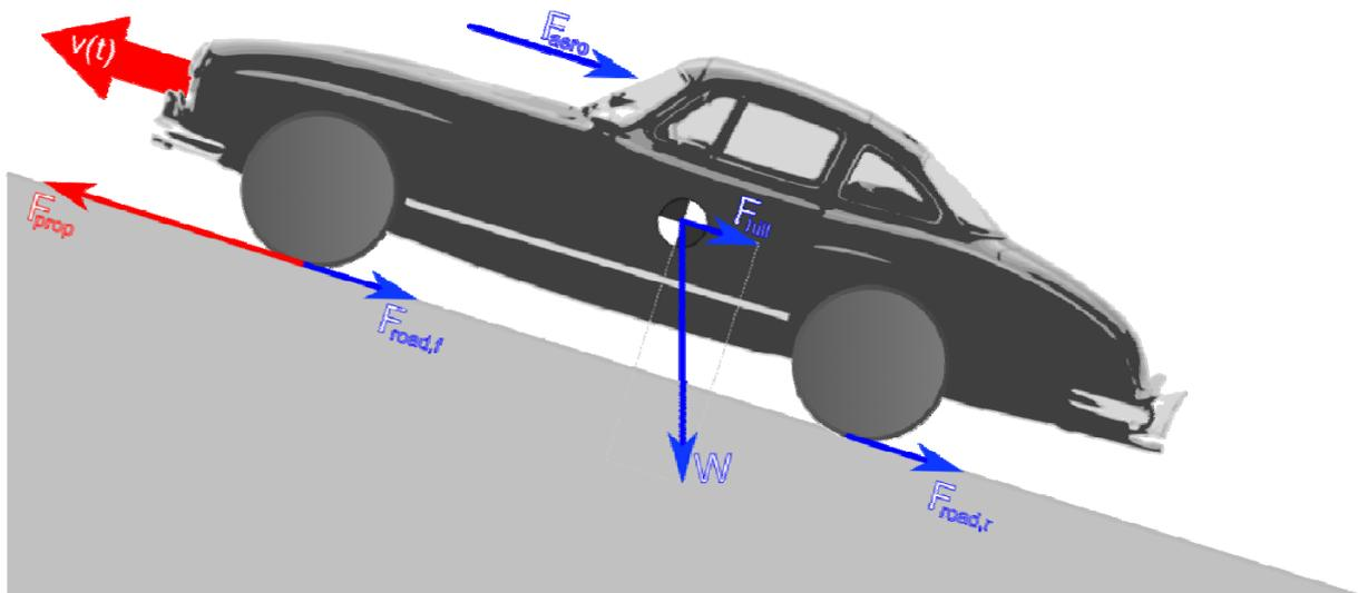
Figure 1: main forces acting on a vehicle going uphill at velocity  $v(t)$
